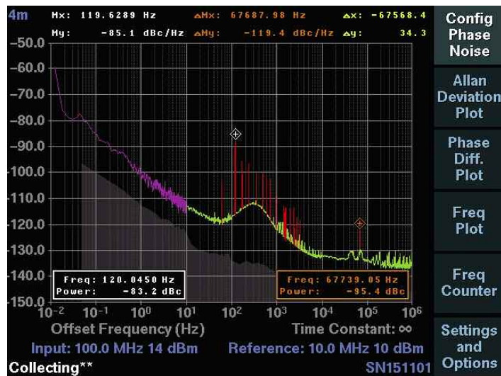
5125A Sample Display Capture – Phase Noise
